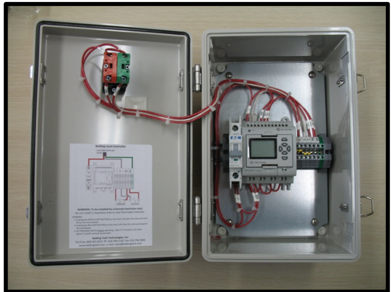
Inside of Belding Level Controller
