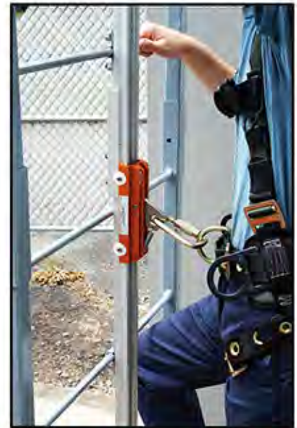
Ladder / Rigid Rail Climbing System in use
